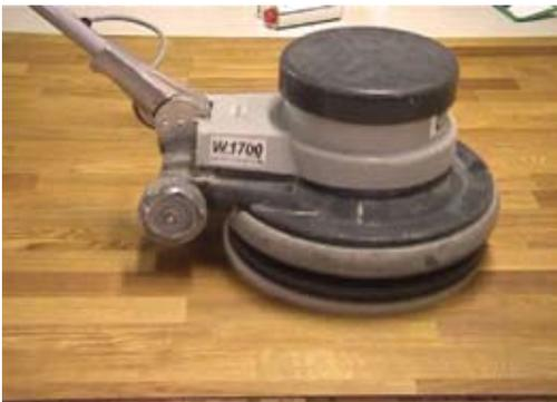
Step 7. Using a white scotch brite pad, buff the material into the floor.
